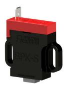
We recommend the brush ride perpendicular to the shaft. The track in which the brush rides on the shaft should be free of scratches, nicks, dents, or defects of any kind. Ideally the shaft surface should be clean with a surface finish within the standard range of most motor manufacturers of 8 to 63 RMS. Do not use any external lubrication. The brush will supply its own extreme lubrication.
