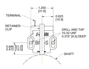
Once the holder is installed **remove** the Brush Retainer Clip used to hold the brush in place. **Connect** one end of the supplied ground wire to the terminal and the other end to ground.
